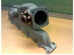
Usually "standard" lead-time for a sand cast aluminium intake manifold is about 2 months. In this case they made 3 different manifolds spending only 6/9 working days. So the engineering phase that usually takes several months, lasted less than 2 weeks!
