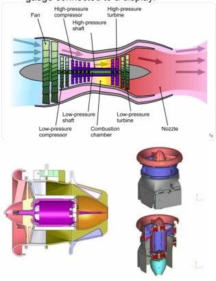
The mini-fan made from WINDFORM® XT for a fluid dynamic study is composed of a mini axial compressor fitted in a case and characterized by high stiffness values, therefore able to minimize those vibrational problems that affect prototypes made of other materials.
