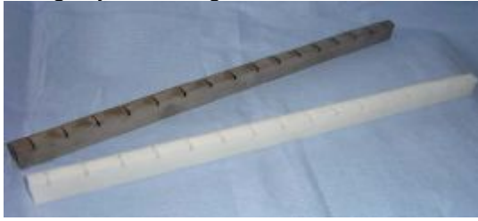
Figure 6: Plated and raw Waveguides made by Stereolithography (Astrium)
