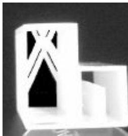
Figure 6: Plated and raw Waveguides made by Stereolithography (Astrium)
