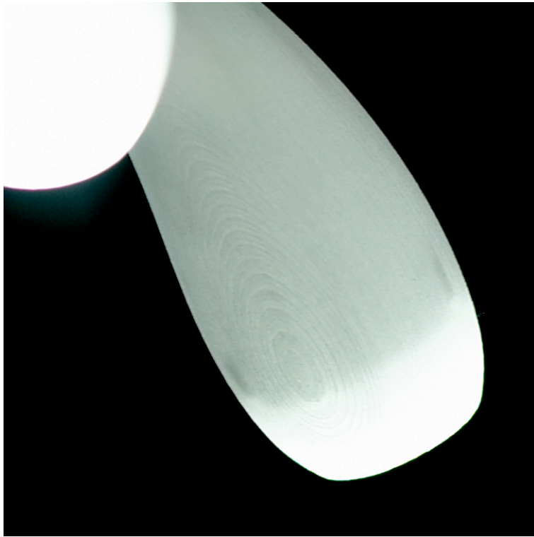
Figure 5: Texture of SLS nylon when lit (FutureFactories, Tuber9).
