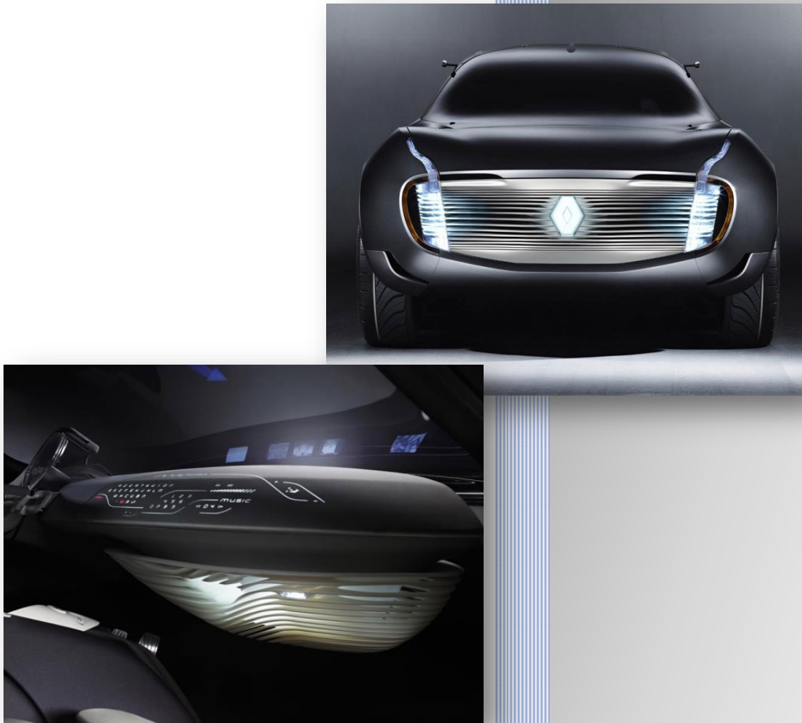
Figure 6: (left) A Laser sintered dashboard by Materialise for the Renault Ondelios concept car (above) (Courtesy of Renault) (Source: http://www.renault.co.uk/about/innovations/ondelios.aspx )
