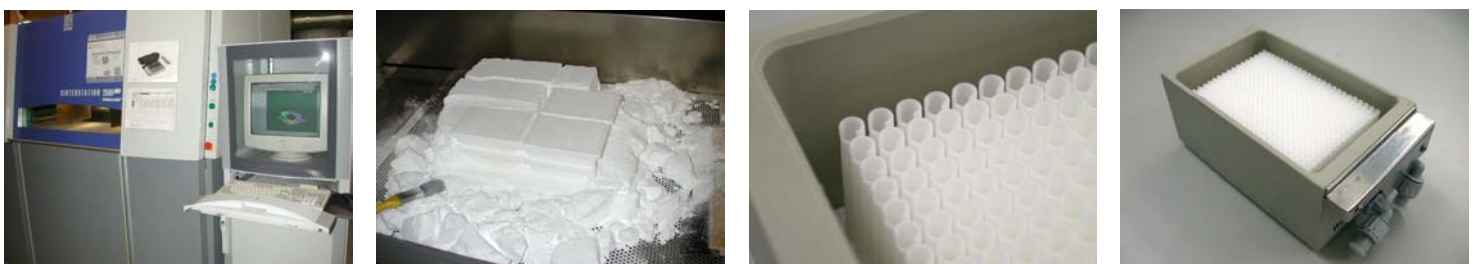
Picture 2: production procedure (laser sintering, unpacking of parts, assambling, end product (pict.: FHS))
