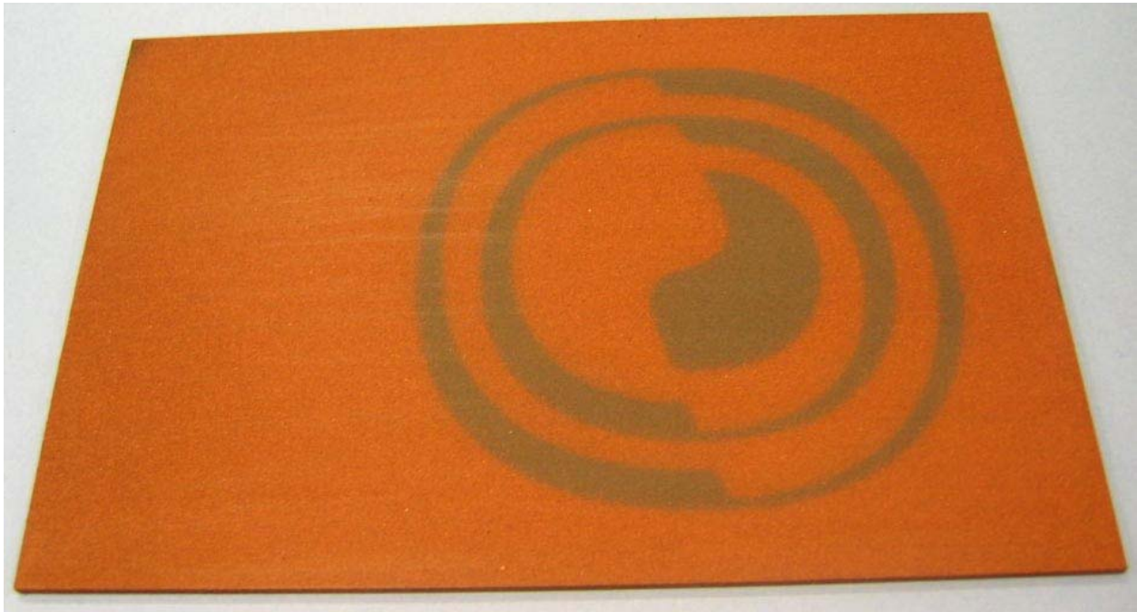
Figure 4. A graphite sheet with copper and iron powder (dark) deposited on it.
