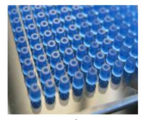
FIG. 3: BATCH WITH RMPD<sup>®</sup> GEARS, MODULE 0,06; DIAMETER 1,2MM AND 0,86MM
