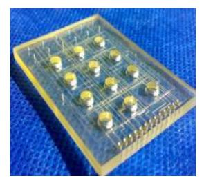
FIG. 2: MICROFLUIDICS WITH TWO FLUIDIC AND CONDUCTOR LEVELS EACH
