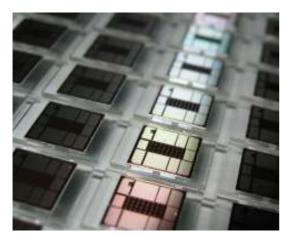
FIG. 6: 3D-CSP BATCH AFTER THE PICK-AND PLACE PROCESS
