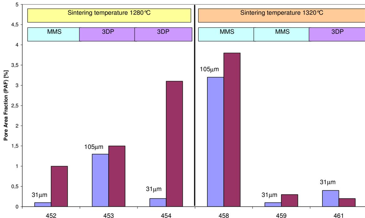
Figure 2: Results of porosity measurement - Pore Area Fraction (PAF)
