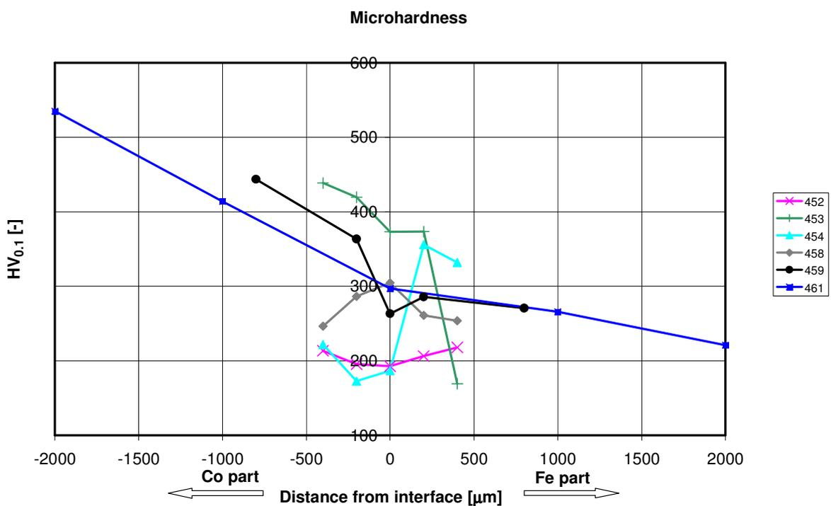
Figure 3: Results of microhardness measurements
