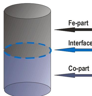
Figure1: Multimaterial sintered sample
