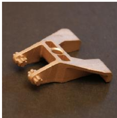
Morris likens the unfinished surface of the DMLS parts to an EDM finish.
