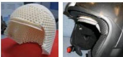
Liner manufactured using additive manufacturing technique
