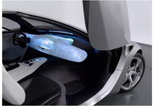
The interior of the car is not conceived as a separate element but is fully integrated with the overall design. The instrument panel is designed as one integrated semitransparent piece, deriving its richness from a sophisticated play of light that serves as a visual and intuitive feedback for the different functions.
