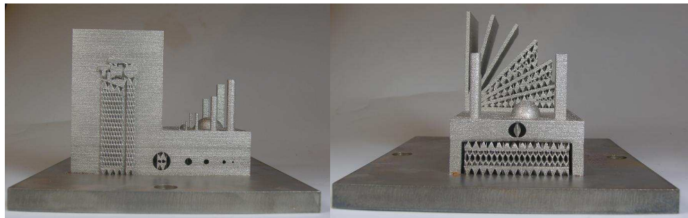
Figure 17 MCP part with supports at left and front plane
