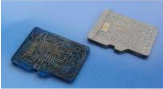
**FIG. 5: MICROSD CARD WITH DIE STACKING**
